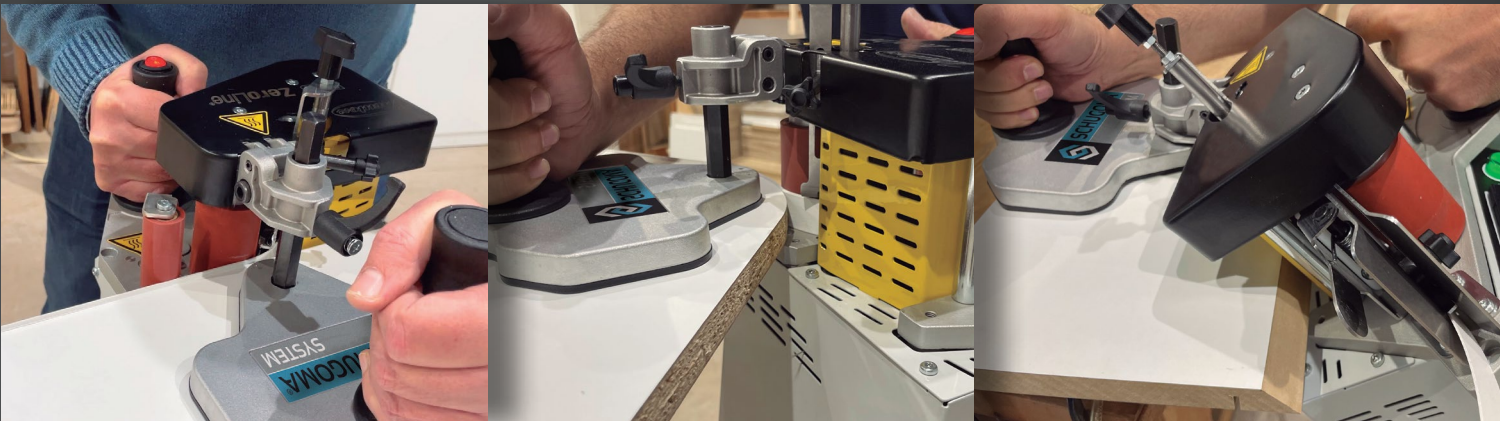
Perfect finishing on straight, round, shaped and inclined panels (0° - 50°)
